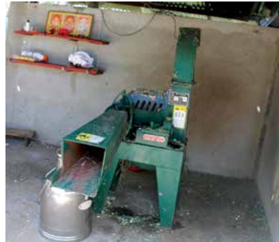
A fodder chopper used by an IHP beneficiary in Oddusuddan for income generation.
